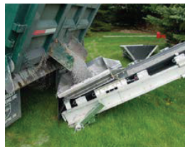
Low profile hopper 1.05 m x 0.9 m (Optional)
