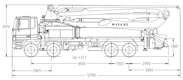
Note: Standard version. Dimensions and weights depend on truck, pump model and equipment. Dimensions in mm, MB-Actros 4144 as example.
