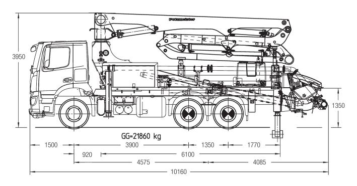
Note: Standard version on 3 axles. Dimensions and weights depend on truck, pump model and equipment. Dimensions in mm, MB-Arocs 2636 as example.
