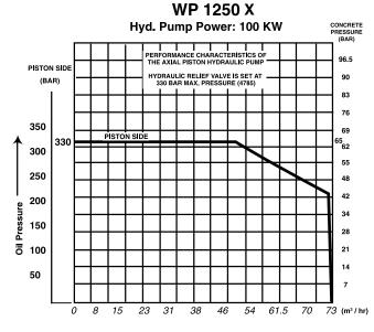
Piston Side 5 10 15 20 25 30 34 (stroke/min) 20 40 60 80 100 120 140 160 180 200 220 240 260 280 Oil Volume (liter/min)
