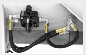
Components, such as a shut-off valve, can be easily operated by the SP 2800 (with up to 210 bar and up to 30 l/min) via the hydraulic control unit.
