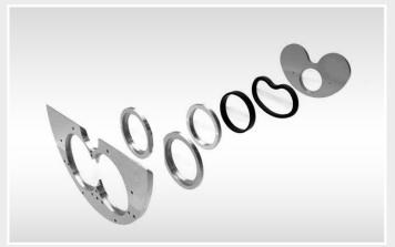
Due to the hardened surface, the carbide wear parts have a significantly longer service life than standard wear parts. As such, the maintenance effort and service costs are reduced, whilst the availability of the SP 1800 is increased.
