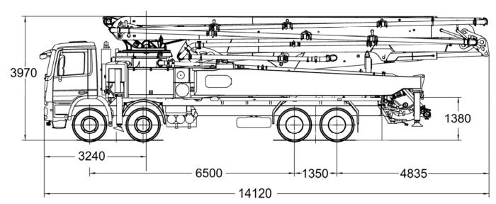
Note: Standard version. Dimensions and weights depend on truck, pump model and equipment. Dimensions in mm, MB-Actros 4640 B, Euro 2. For illustration only.
