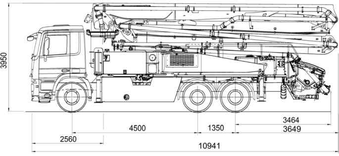
Note: Standard version. Dimensions and weights depend on truck, pump model and equipment. Dimensions in mm, MB-Actros 2632 Euro 5 as example. For illustration only.
